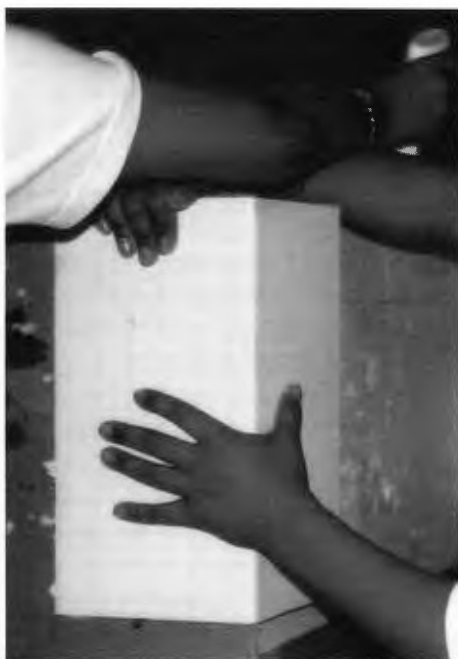
4-45: Adding cardboard flap to strengthen back-to-side joint
