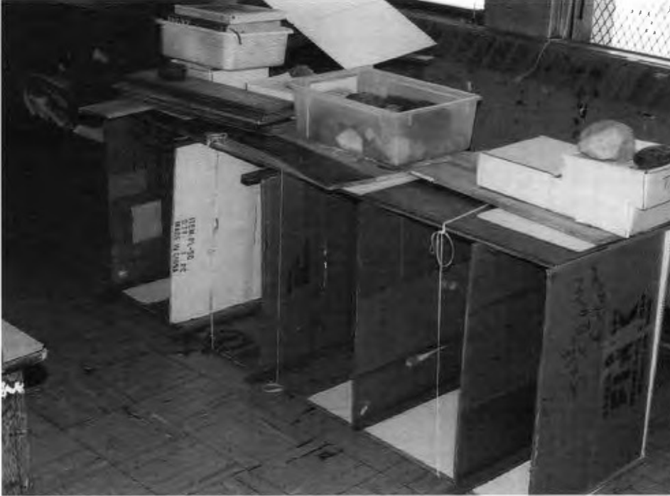
4-42: Gluing the sides to the back, using the shelves to keep things in place
