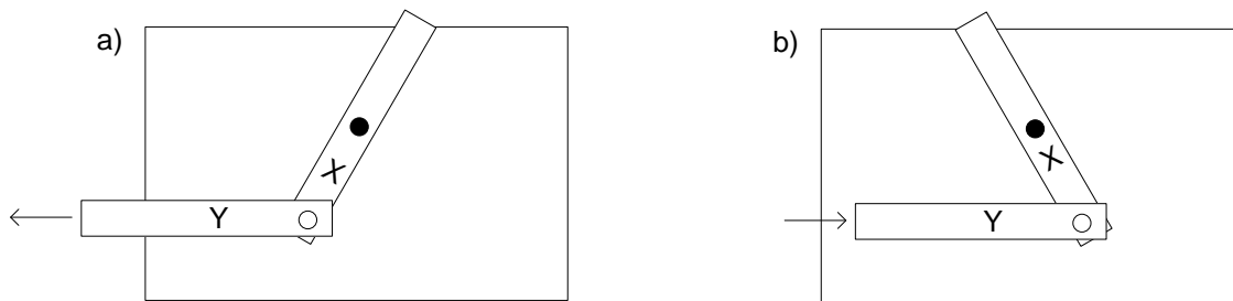
Figure 5: Strip Y now controls strip X
