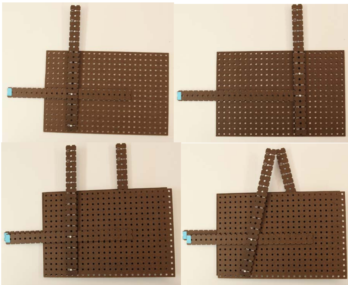
Figure 6: Two one-output mechanisms (top) are placed one on top of the other (bottom left), and then operated in tandem to work like a two-output mechanism (bottom right)
