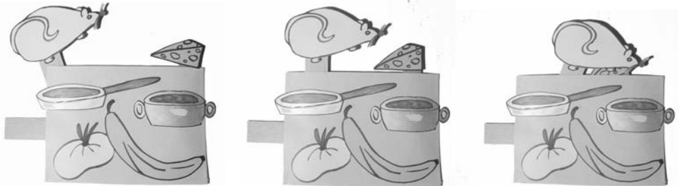
Figure 2: Mouse MechAnimation, showing output motion as input moves to the right
