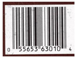
Each number is represented by seven strips, each of which could be white or black. A white stripe reads as binary 0, while a black stripe represents binary 1. The codes are different on the left and right sides. The longer pairs of stripes at the left, right and center are called "guard bars," which tell the scanner when to start, stop and switch from left to right. The code for each number, on the right and the left, are shown in the translation table on p. 3.
