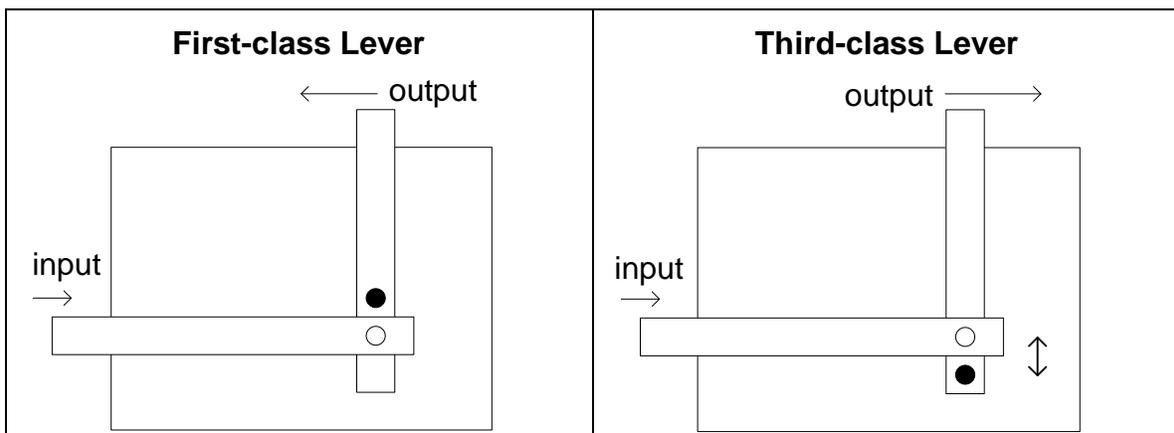
Key: ○ Fixed pivot (attaches strip to base)
