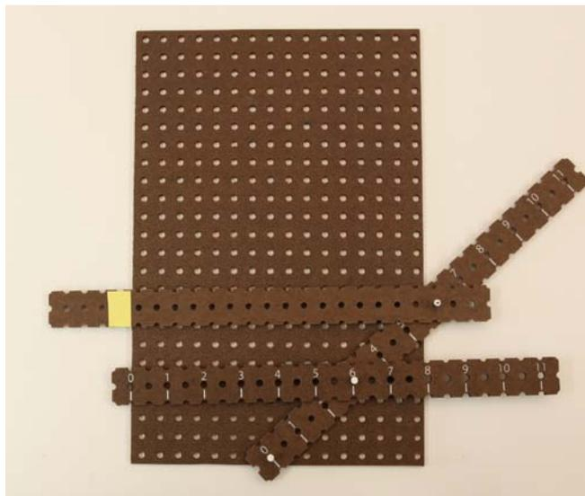
d) Place the 0 " hole of the vertical lever over the fixed pivot. Move the input link so the 0 " mark lines up with the left edge. Keep input and output arms parallel to the holes in the base. Mark the output link with a Post-it™ or tape, even with the left edge of the base. This is the starting position.
