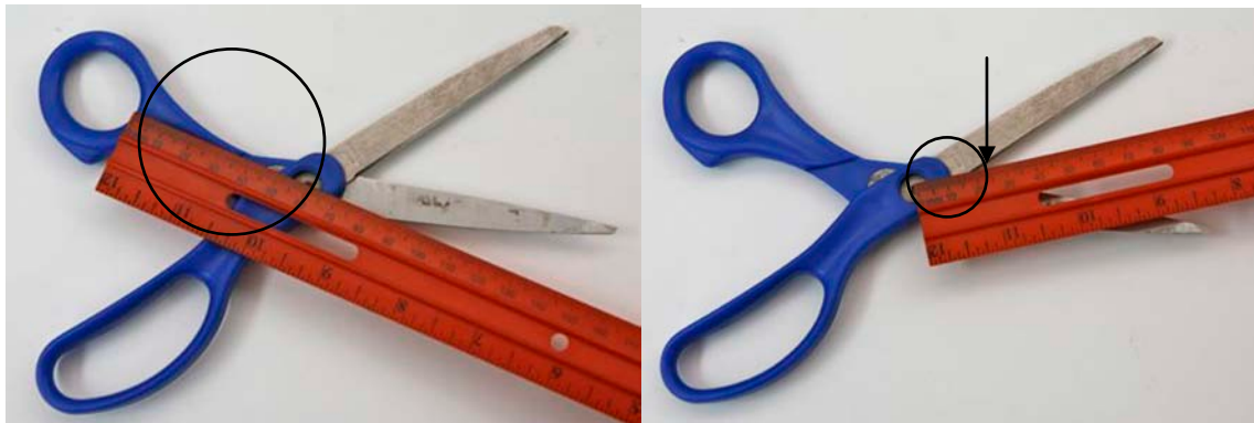
Figure 1: Input arm, from input to about 60 mm
